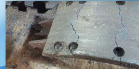
OUT OF SERVICE PORTION OF LINING MISSING THAT EXPOSES A FASTENING DEVICE
